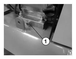
Remove the oil drain plug (1)
